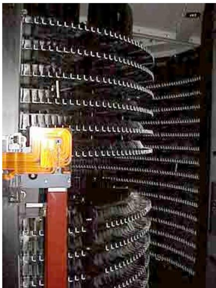
Figure 2. The Powderhorn Robot has room for 6000 tape cartridges with capacities up to 200 gigabytes each. As such the total capacity of this system can be more than 1 petabyte (1,000,000,000,000,000 bytes).
